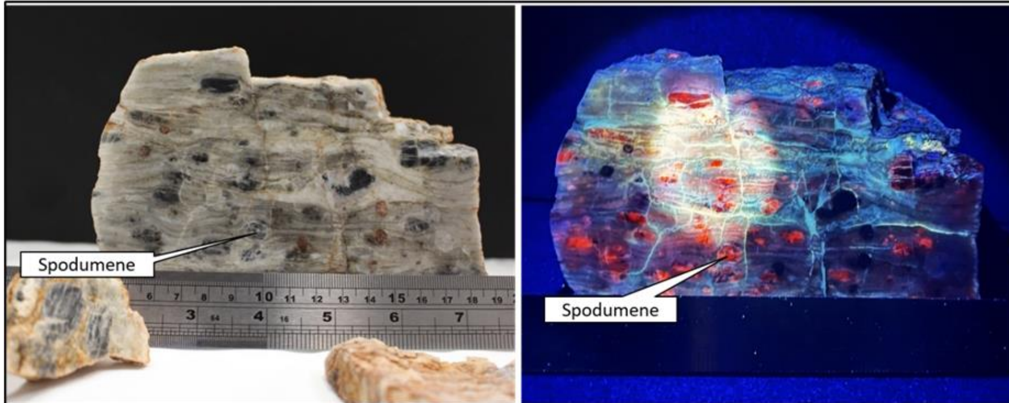
Prinsep spodumene bearing pegmatite sample under white and UV light – spodumene has an orange fluorescence
