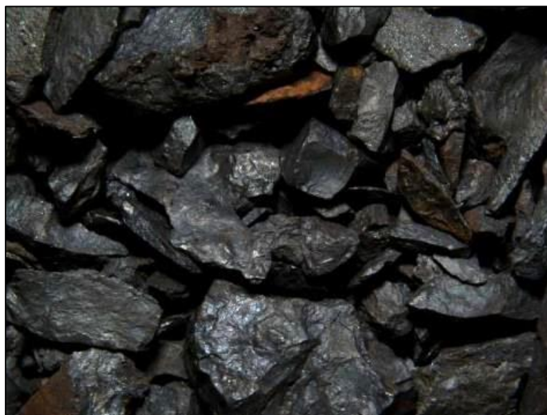
Figure 3: Photograph of the Braeside West prospect Heavy Media Separation bulk sample material
