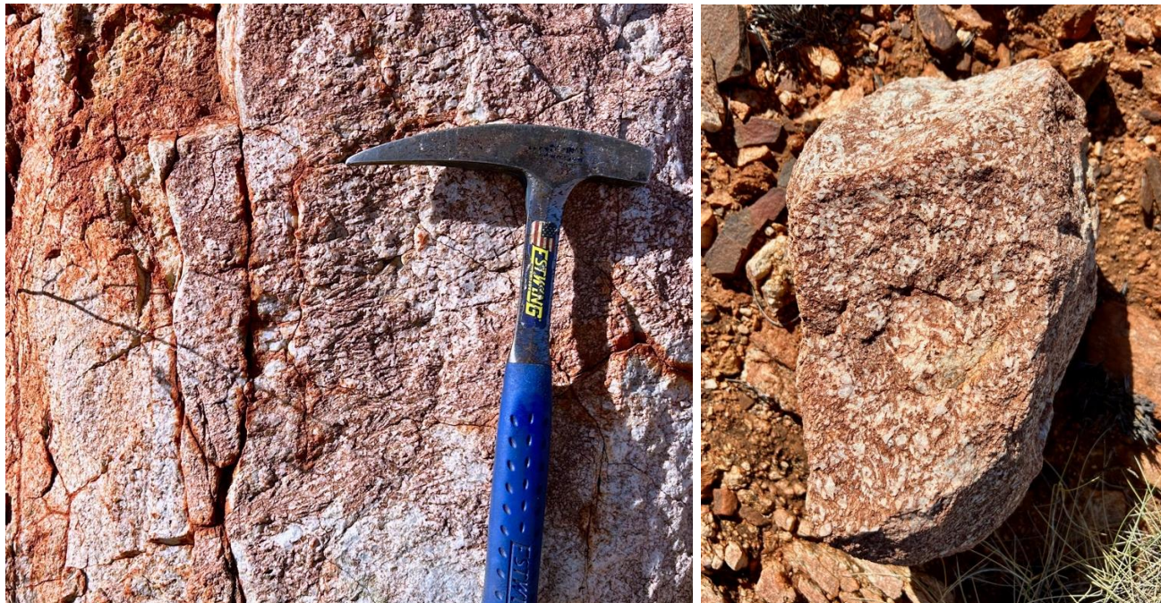
Figure 2: Outcrops from Prinsep northern zone with weathered semi spinifex textured lithium mineralisation
