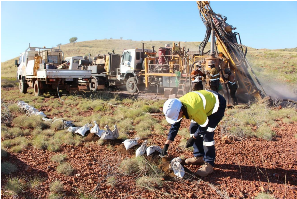
Figure2 – Drilling at Woodie Woodie North Manganese Project, Barramine Prospect
